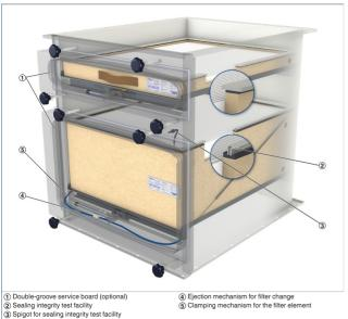
Ducted particulate filters KSFS for critical requirements as filter casings for installation into the ductwork of ventilation systems.
