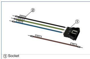
② Text label carrying the ID of the terminal on the TCU3 main PCB and on the PCB of the EM-TRF or EM-TRF-USV
