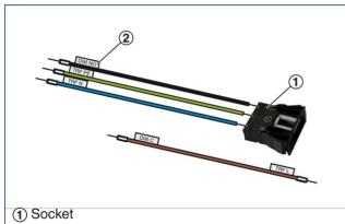
② Text label carrying the ID of the terminal on the TCU3 main PCB and on the PCB of the EM-TRF or EM-TRF-USV
